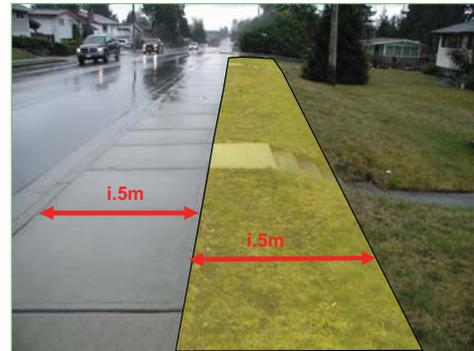
*Image shows existing 1.5 metre wide sidewalk and proposed new multi-use pathway width.*
