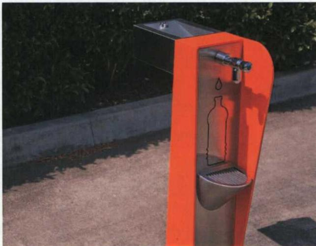
Fig.98 Example of drinking water station with bottle filler and bubbler
