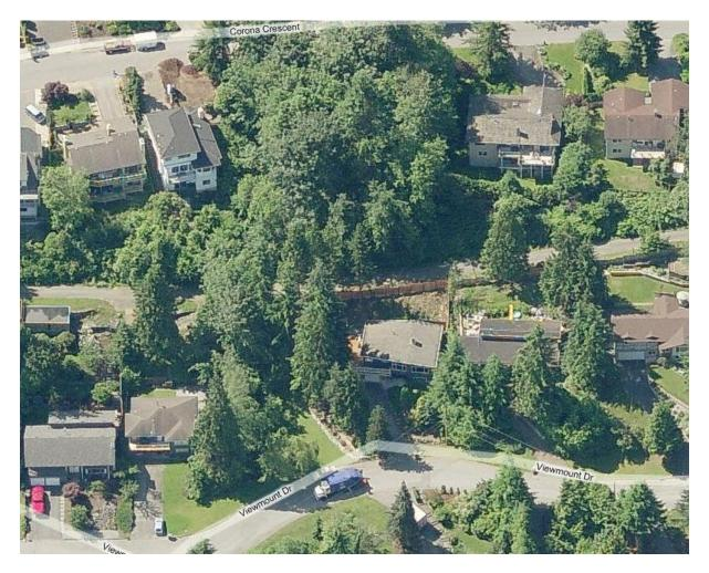
Photo 6: View over future debris flow track, pre 2009. The future headscarp is about at top centre. Some deciduous and evergreen trees were removed by the failure, with most depositing on a paved lane in the centre of photo. Photo from Bing Maps.
