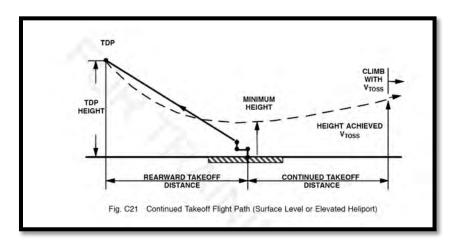
There are trade-offs in Category "A" procedures for every helicopter type. Although the EC135T2 in the previous drawing can climb to a significant height and help clear obstacles in its path, rearward clearance is a requirement – something that is not in abundance at the CFR heliport.
