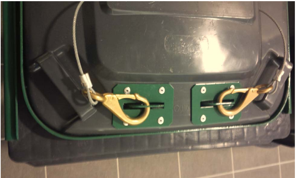
Top view of 120L cart showing current bear-resistant hardware installed.
